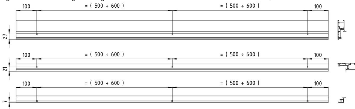
Fig. 9. Diagram for drilling the mounting holes in the guide profile and the guide revision profile.
